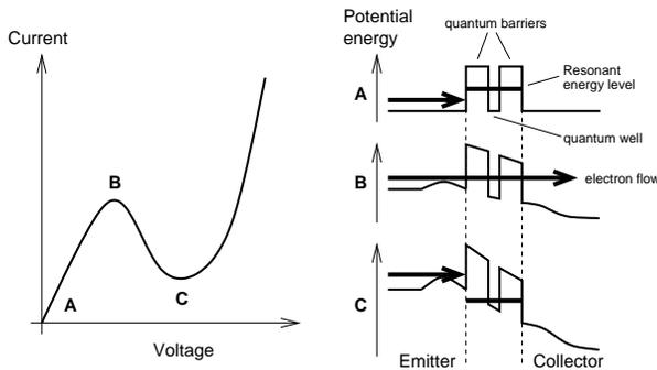
Figure 1.  $I$ - $V$  characteristics and energy band diagrams of the resonant tunneling diode.
